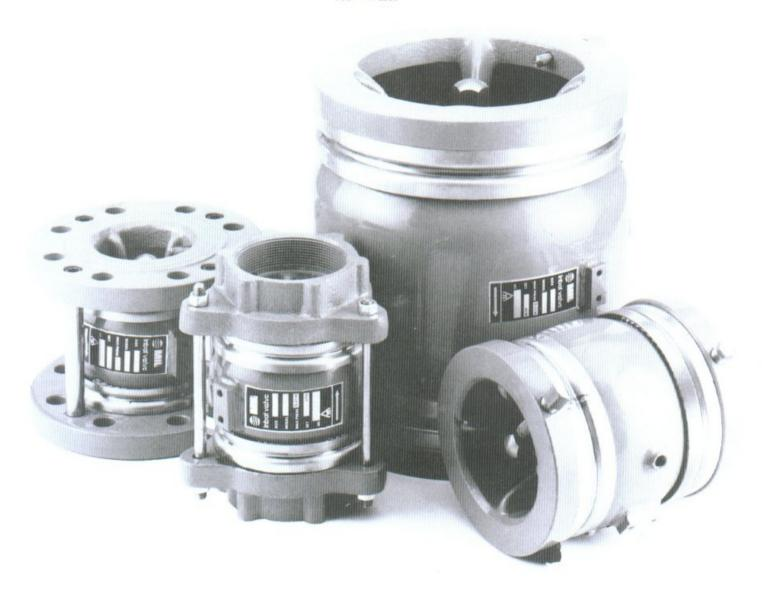
The **Inbal** series 700 is a pressure operated, sleeve actuated, in line, axial valve, designed for heavy duty conditions. It consists of four major components: The valve housing, the sleeve assembly, the core and the ends. The sleeve assembly is the only moving part.
